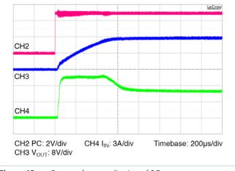
**Figure 13** — Start up from application of PC;  $V_{IN}$  pre-applied  $C_{OUT} = 800 \mu F$
