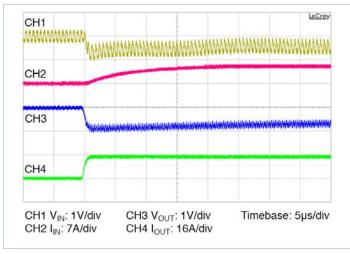
**Figure 14** — 0A - 15A transient response:  $C_{IN} = 330\mu F$ ,  $I_{IN}$  measured prior to  $C_{IN}$ , no external  $C_{OUT}$
