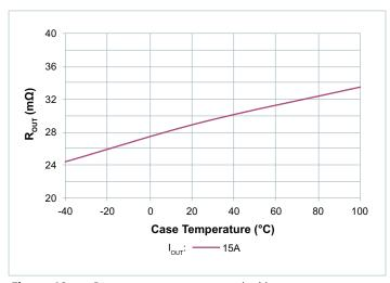
**Figure 10** — R<sub>OUT</sub> vs. temperature; nominal input
